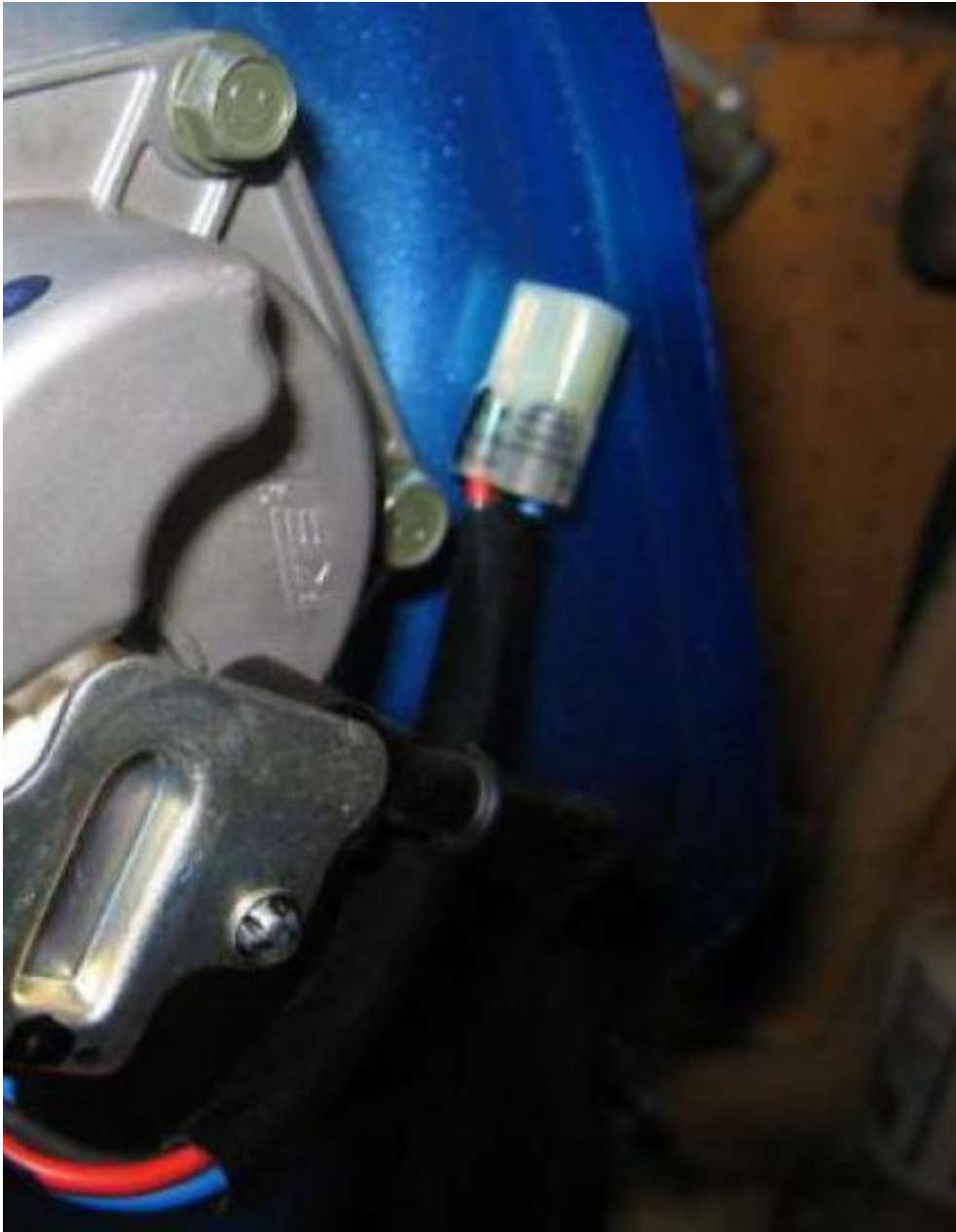
The fuel pump electrical connector simply unclips (small screwdriver) and pulls apart.
