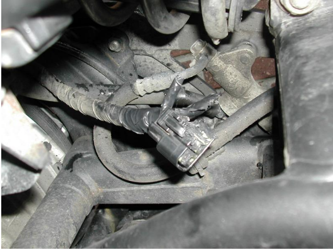
Damaged Regulator/Rectifier Loom Plug
